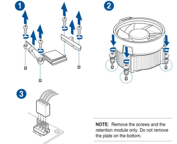
NOTE: Remove the screws and the retention module only. Do not remove the plate on the bottom.
